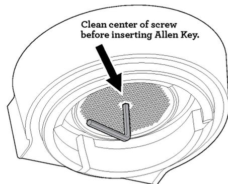
5. Once loosened, carefully remove and retain the screw and the stainless steel shower screen. Make note of the side of the shower screen that is downwards. This will make re-assembly easier. Wash the shower screen in warm soapy water, then dry thoroughly.
