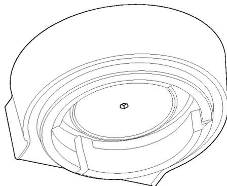
7. Re-insert the shower screen, then the screw. With your fingers, turn the screw clockwise for 2-3 revolutions then insert the Allen Key to tighten until the screw is flush with the shower screen. Do not overtighten screw.
