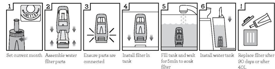
The provided water filter helps prevent scale build-up in and on many of the inner functioning components. Replacing the water filter after three months or 40L will reduce the need to descale the machine.
